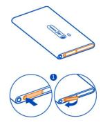
2 To unlock the SIM card holder, slide the holder to the left. Carefully pull out the holder.
